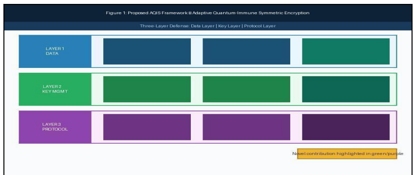
Fig 3: Three-layer AQIS architecture. Layer 1 handles data encryption. Layer 2 manages quantum-safe session keys and AKRP rotation. Layer 3 defines the PCACS-PQC handshake protocol
