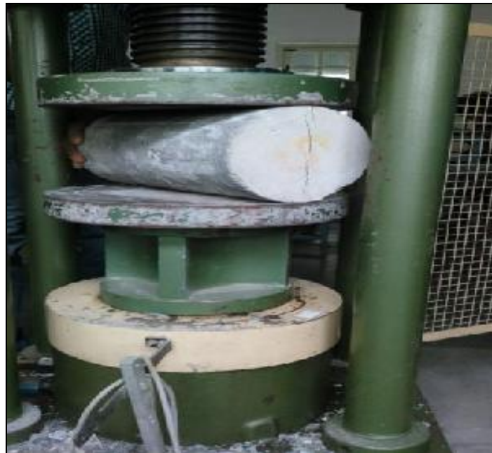
Photograph 3 Testing of specimen (split tensile strength test)
