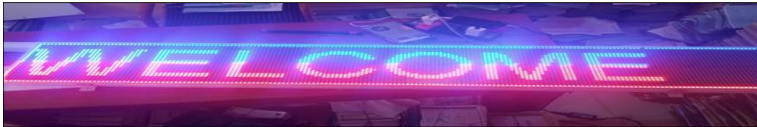
Fig 3: 5 x 7 LED panel displaying the word welcome without spacing
